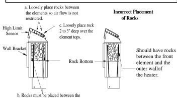
1. Put smaller rocks in first around the outer perimeter of the rock compartment.
